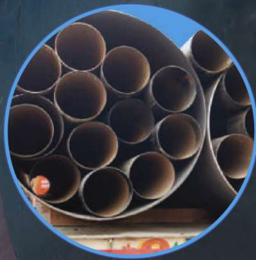
TELESCOPIC NESTING OF PIPES
